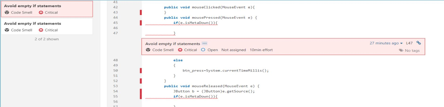
The screenshot shows a code editor with two instances of the 'Avoid empty if statements' code smell. The first instance is on line 45, and the second is on line 55. A tooltip for the second instance is visible, showing the smell name, severity (Critical), and other details.
